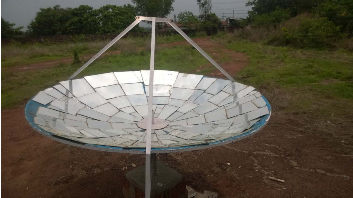
Fig: parabolic dish installed
